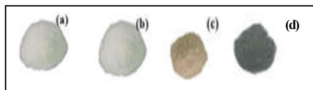
Fig. 1 Preparation of (a) ZnO without annealing, (b) ZnO, (c) ZnO:SnO 2 and (d) ZnO:NiO nanocomposites annealing with 400°C.
